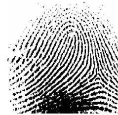
Fig. (8). The fingerprint image after binarization.
