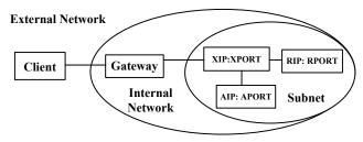
Fig. (5). The network structure of authentication server.
