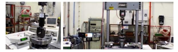
Fig. (4). Magneto-rheological damper with current supply device connected to MTS universal setup.
