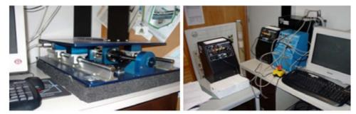
Fig. (5). Quanser shaking table II (and its controllers) at FEUP – Covicocepad Lab.
