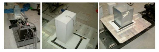
Fig. (2). The shaking table and the rigid blocks used during experiments.
