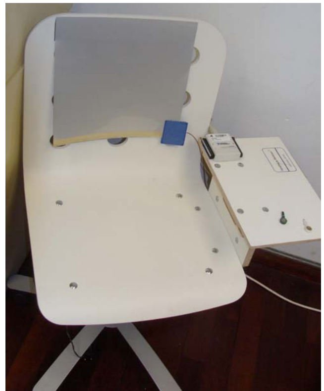
Fig. (7). Prototype described in [58], implementing skin conductivity and ballistocardiogram acquisition and processing.
