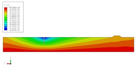
Fig. (5). Cross section of vertical deformation contours.
