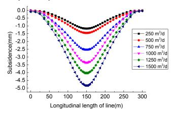
Fig. (8). Influence of pumping rateon subsidence of embankment.
