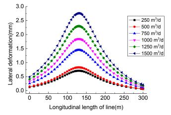
Fig. (9). Influence of pumping rateon lateral deformation of embankment.
