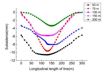
Fig. (10). Influence of pumping distance on subsidence of embankment.
