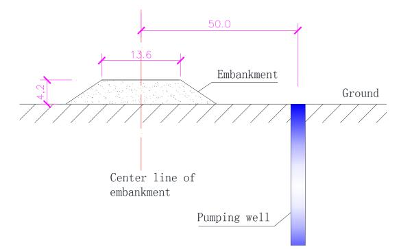
Fig. (1). Relationship between embankment and pumping well (unit:m).
