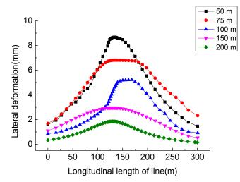
Fig. (11). Influence of pumping distance on lateral deformation of embankment.
