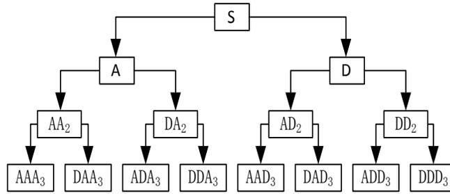
Fig. (1). Wavelet packet decomposition.
