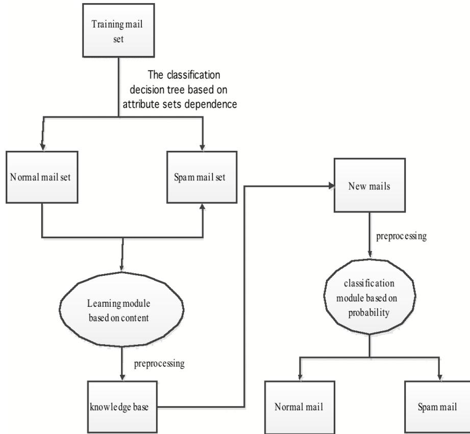
Fig. (2). Process of spam filtering based on Bayesian.
