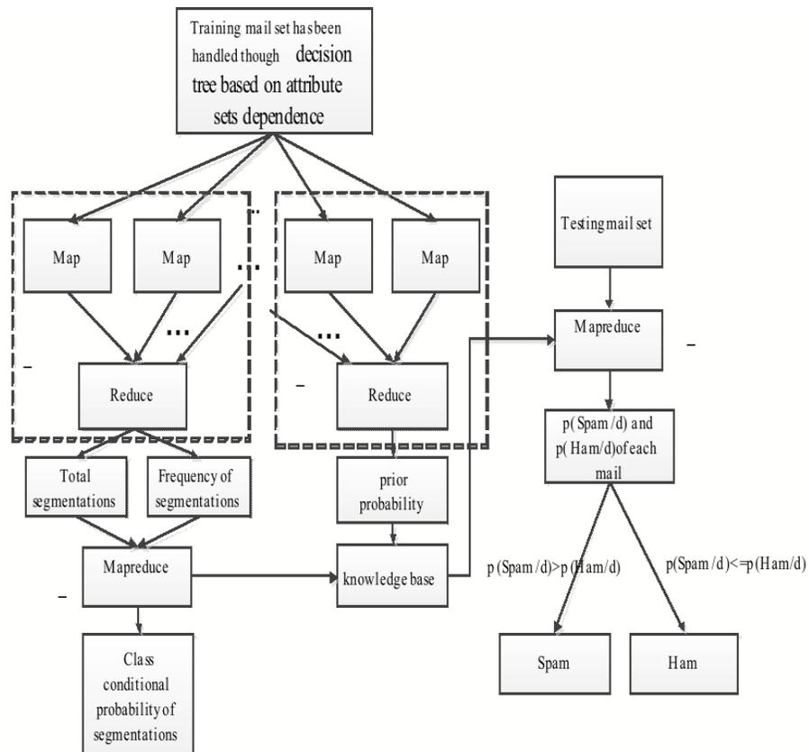
Fig. (3). Bayesian spam filtering mechanism of the decision tree is based on the attribute sets dependence.
