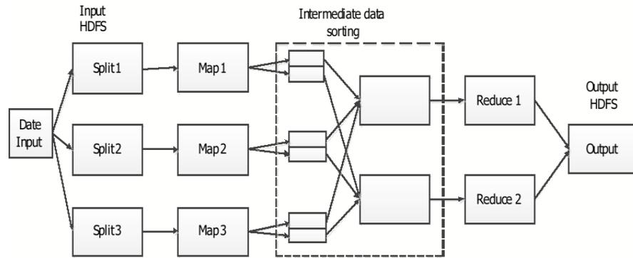
Fig. (1). Operation process of Mapreduce.
