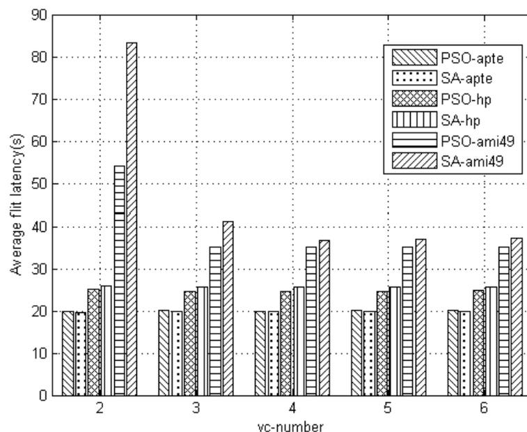
Fig. (2). Comparison of average flit latency for *apte*, *hp* and *ami49* while changing the number of virtual channels from 2 to 6.
