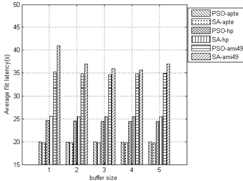
Fig. (5). Comparison of average flit latency for apte, hp and ami49 while changing the size of buffers from 1x to 5x.
