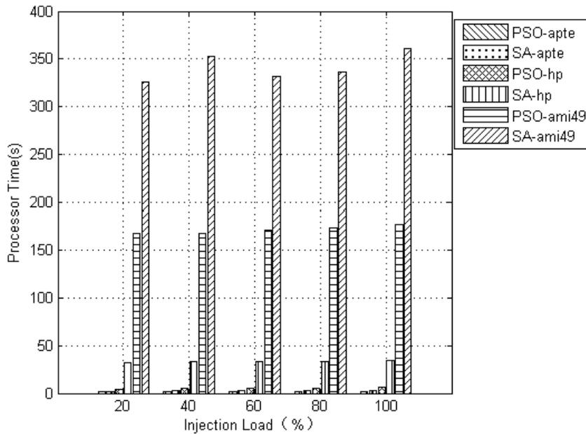
Fig. (9). Comparison of CPU processing time for *apte*, *hp* and *ami49* while changing injection load.
