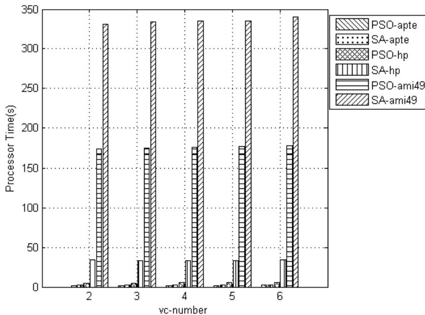
Fig. (4). Comparison of CPU processing time for *apte*, *hp* and *ami49* while changing the number of virtual channels from 2 to 6.
