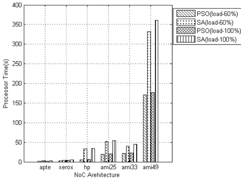
Fig. (12). Comparison of CPU processing time of architectures with different Mesh size when injection load is 60% and 100%.
