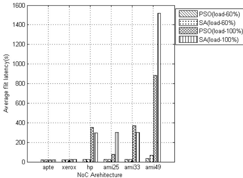
Fig. (10). Comparison of average flit latency of architectures with different Mesh size when injection load is 60% and 100%.
