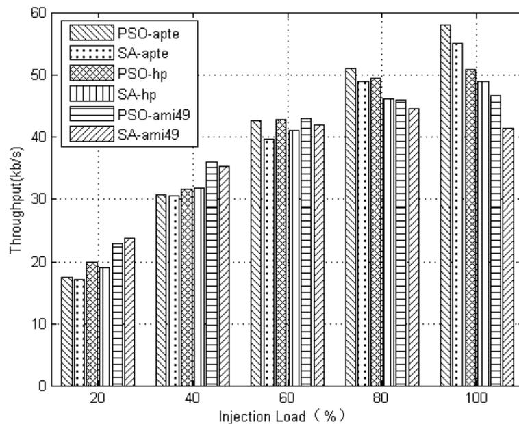
Fig. (8). Comparison of throughput for apte, hp and ami49 while changing injection load.
