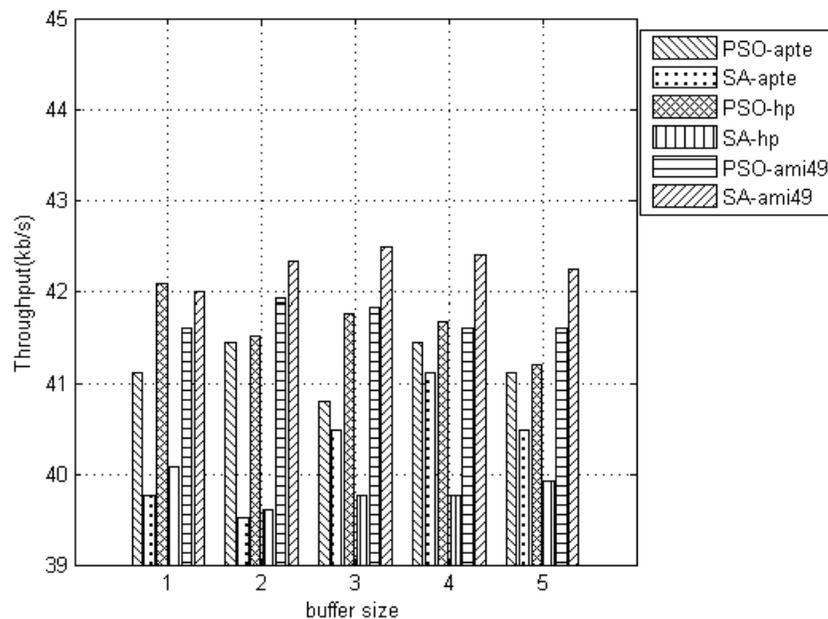
Fig. (6). Comparison of throughput for apte, hp and ami49 while changing the size of buffers from 1x to 5x.
