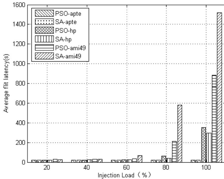
Fig. (7). Comparison of average flit latency for apte, hp and ami49 while changing injection load.
