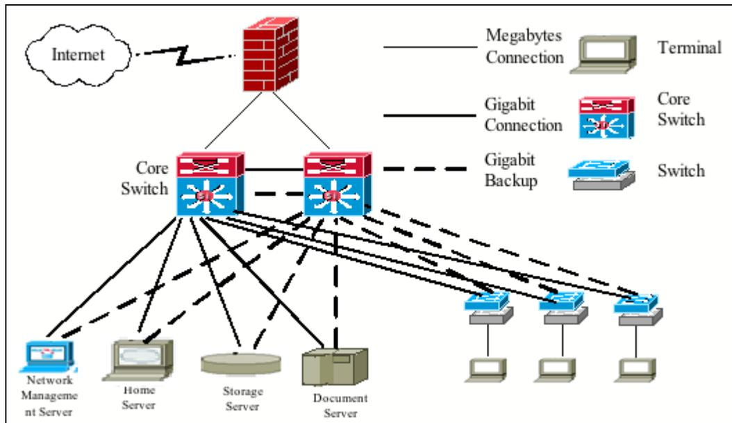
Fig. (4). Backbone network topology figure.
