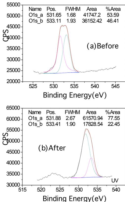
Fig. (5). XPS of O1s in AEROSPACE white paint before and after exposed to UV irradiation.
