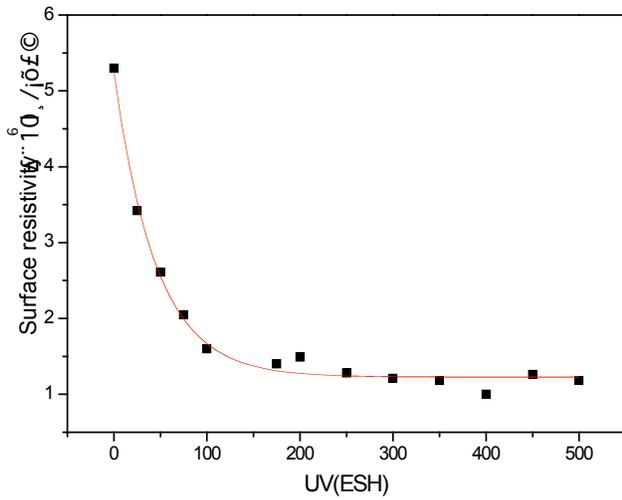
Fig. (1). Fitting surface resistivity versus irradiation time.
