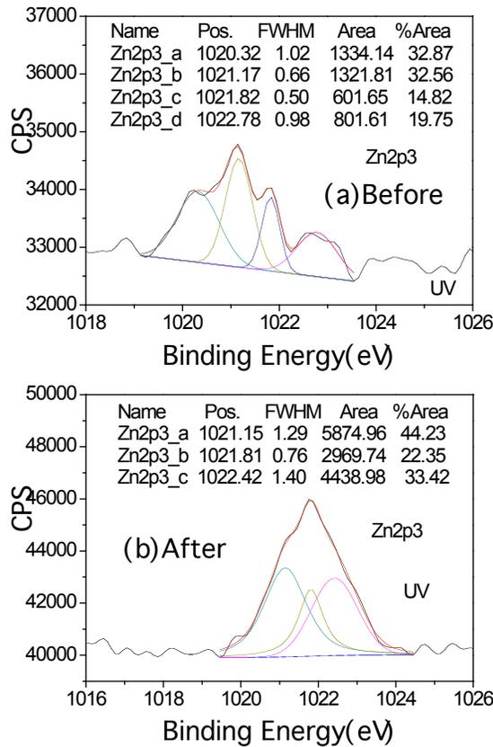
Fig. (4). Energy spectrum of Zn2p3 in AEROSPACE white paint before or after irradiated near UV irradiation.
