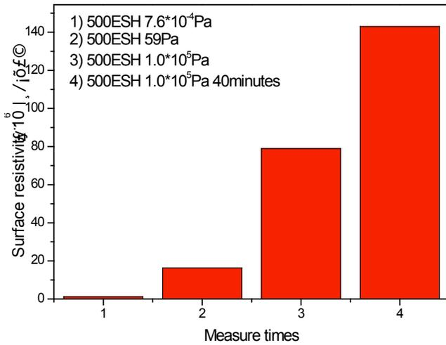
Fig. (2). Surface resistivity of AEROSPACE white paint versus pressure.
