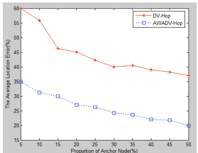
Fig. (6). The average location error with wormhole attack.
