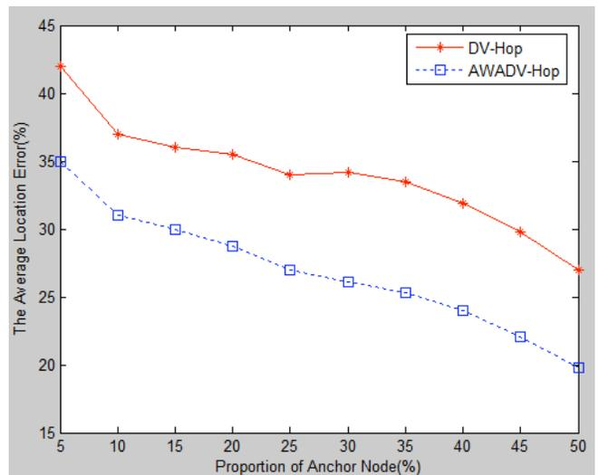
Fig. (5). The average location error without wormhole attack.
