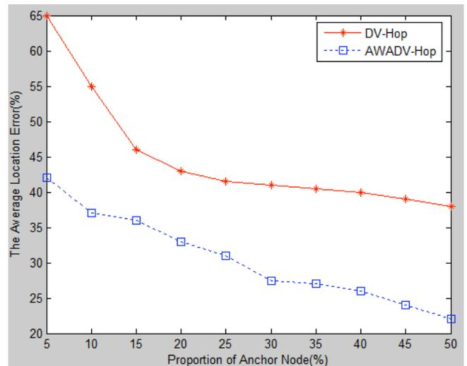
Fig. (4). The average location error with wormhole attack.
