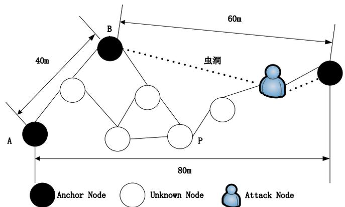
Fig. (1b). DV-Hop suffering wormhole attack.
