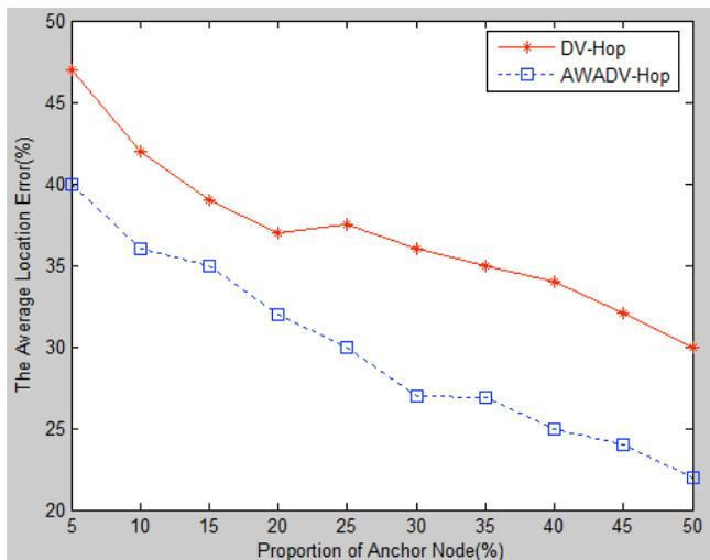
Fig. (3). The average location error without wormhole attack.
