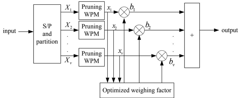
Fig. (7). Block diagram of PTS technology based on pruning WPM and improved threshold search method at sending end.
