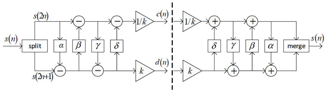
Fig. (2). Implementation of lifting wavelet transform and inverse lifting wavelet transform.
