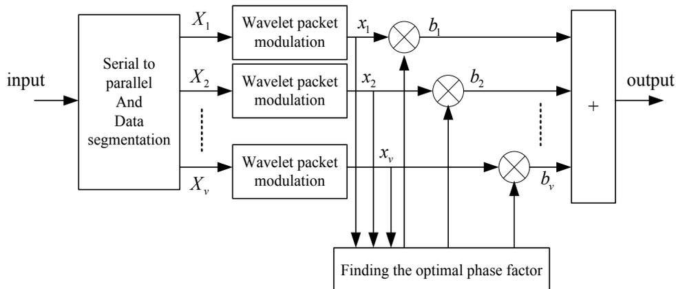
Fig. (5). Block diagram of PTS technology at sending end.
