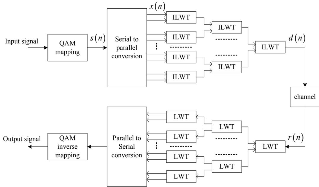
Fig. (1). Block diagram of wavelet packet multicarrier modulation system based on lift scheme.
