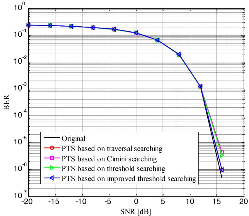
Fig. (10). Comparison of BER for PTS based different search methods.
