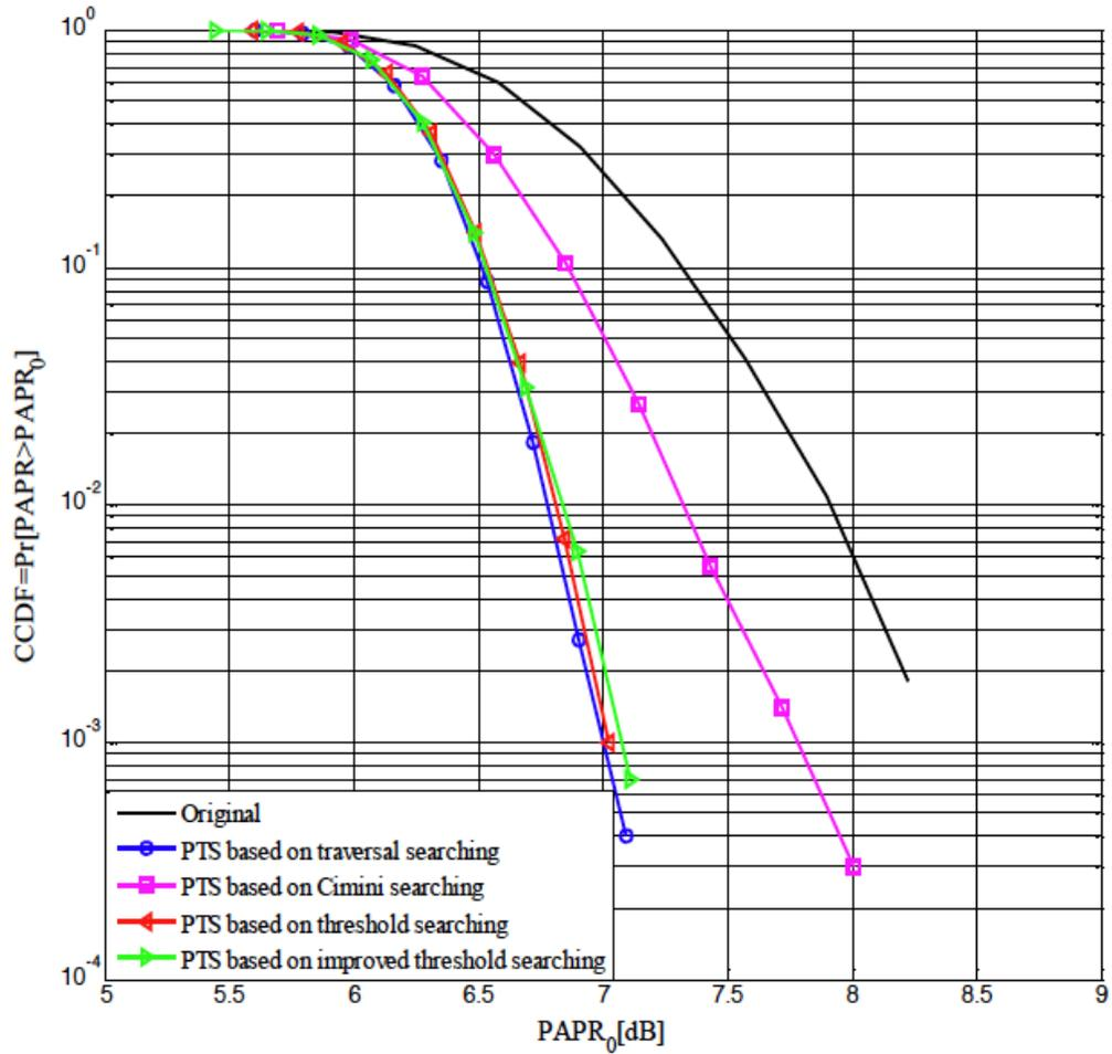
Fig. (9). Comparison of the distribution curves of PAPR for PTS technology based on different search methods.
