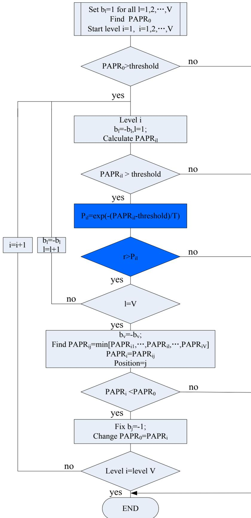
Fig. (6). PTS algorithm based on improved threshold search method.
