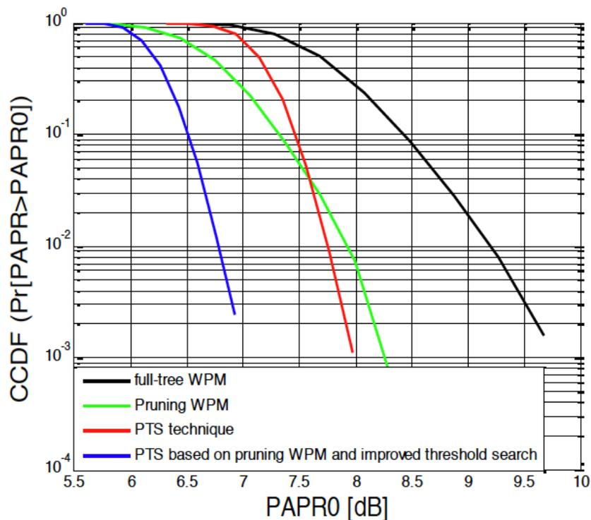
**Fig. (11).** Comparison of the distribution curves of PAPR for different schemes.
