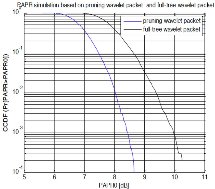
Fig. (8). PAPR simulation for LOWPM system based on pruning wavelet packet and full-tree wavelet packet.
