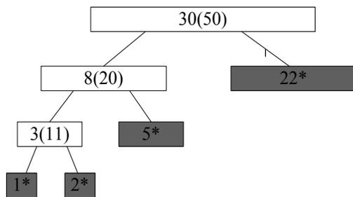
Fig. (4). The optimal wavelet packet tree structure (pruning wavelet packet).
