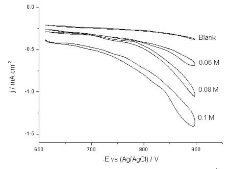
Fig. (1). Cyclic voltammograms of the background electrolyte and that of formic acid 0.06, 0.08 and 0.1 mol L<sup>-1</sup>. Scan rate 5 mV s<sup>-1</sup>.
