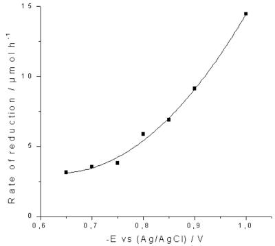
Fig. (2). Rate of the reduction of HCOOH against the cathodic potential, in a 2 mol  $L^{-1}$  HCl solution. Electrolysis time 120 min.
