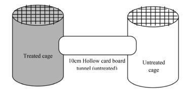
Fig. (1). Set up for repellence evaluation using the cage assay method (Bigoga model).
