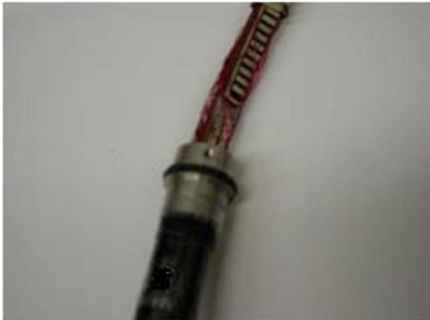
**Fig. (2).** Serial connection of 15 bending sensors on both sides of a substrate in the shaft of the colonoscope.
