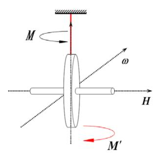
Fig. (3). Maglev gyro north measurement schematic.
