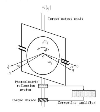
Fig. (4). Photoelectric torque feedback control principle.
