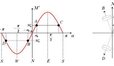
Fig. (5). Two-position north-seeking principle.
