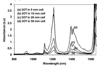
Fig. (6). NIR absorbance spectra of the 3OT monomer.
