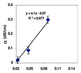
**Fig. (5).** Attenuation coefficient of P3HT solution versus the molar ration of polymer in solution.
