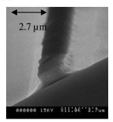
Fig. (10). Two SEM images of the first ridge based on synthesized RIRg P3OT.
