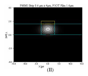
**Fig. (11).** (I) Schematic representation of created P3OT SLWG. (II) Dimensions and intensity profile for a singlemode P3OT SLWG.
