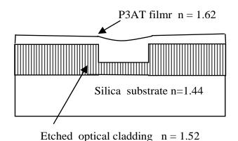
Fig. (12). Cross section of a buried waveguide.
