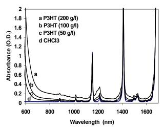
Fig. (4). NIR absorbance spectra of CHCl<sub>3</sub> and purchased P3HT in CHCl<sub>3</sub> solutions for different ranging concentrations.
