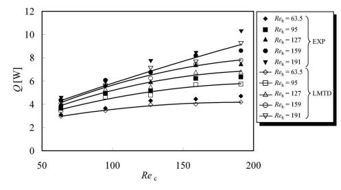
Fig. (7). Prediction of heat transfer rate using the log-mean temperature difference method.
