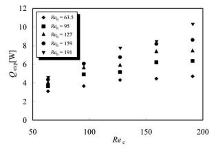
Fig. (6). Heat transfer rate of the parallel flow microchannel heat exchanger.
