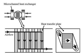
Fig. (4). Schematic view of the airflow.
