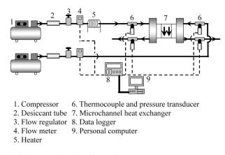
Fig. (1). Schematic view of experimental setup.
