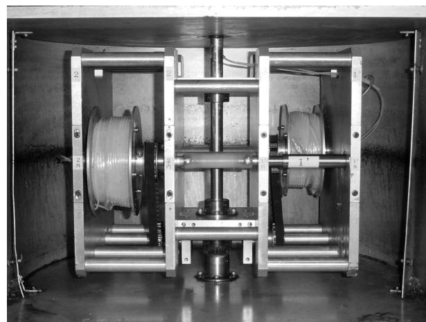
Fig. (3). Photograph of type XL cross-axis coil planet centrifuge.
