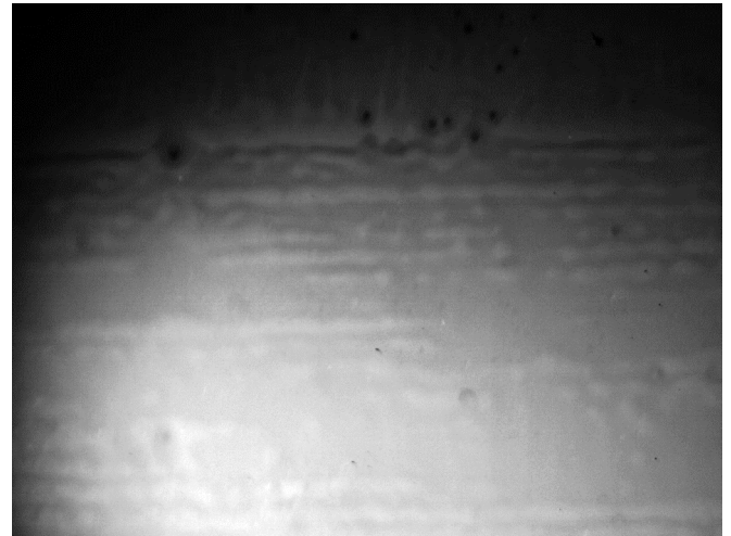
Fig. (6). Motor oil emulsions; lines are motor oil trapped in standing waves at 2.253MHz in curved cuvette.
