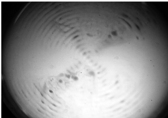
Fig. (2). Oil droplets captured in standing waves concentrically at 1.67 kHz frequency modulated in cylindrical piezo transducer.
