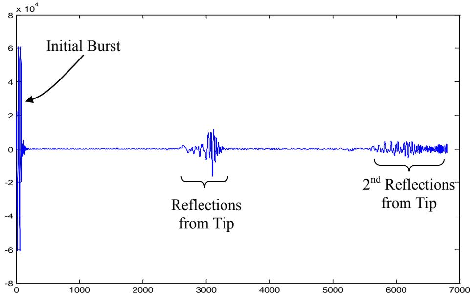
**Fig. (13).** A typical A-line (at 5 MHz) showing the initial burst and two reflections from the tip. The amplitude of the plot is determined by adding the pressure across the tip, and the horizontal axis corresponds to time.
