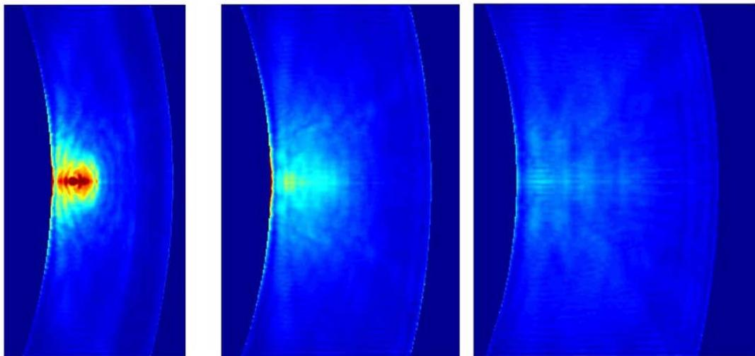
**Fig. (12).** Horizontal slices showing the acoustic energy distribution are shown at shallow, medium, and deep depths into the periodontal anatomy. The curved surface of the tooth is at the left so that the  $z$ -axis of Fig. (6) is now out of the page.
