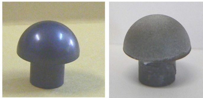
Fig. (7). Hemispherical sample before (left) and after testing (right).
