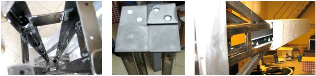
Fig. (14). (left) AISI 316L frame; (centre) UHTC tile installation; (right) Al 2 O 3 tile installation.
