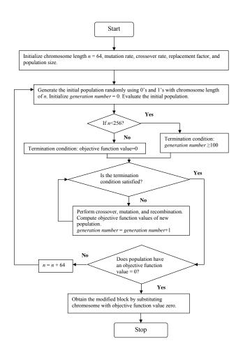
Fig. (6). The variable- length chromosome procedure.
