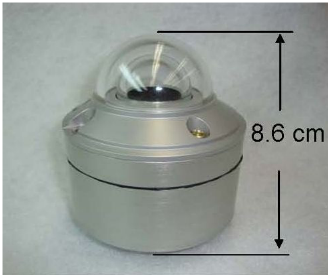
Fig. (1). Side view of the modified Kipp and Zonen CM-22 radiometer used for RACORO.
