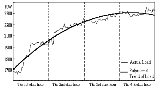
Fig. (8). Load trend is varied by the school class hours at NKFUST.
