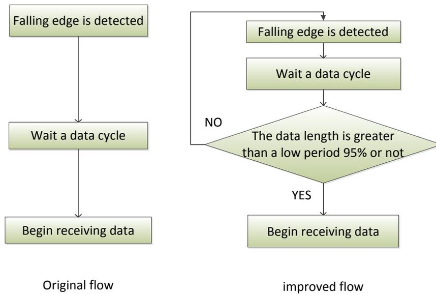
Fig. (7). Change the program flow before and after contrast (fragment).
