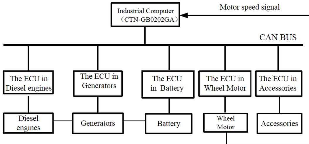
Fig. (2). The diagram of driving system in middle-power electric tractor.
