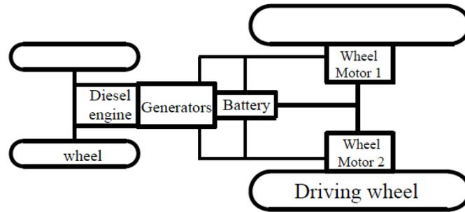
Fig. (1). The diagram of driving system in middle-horsepower electric tractor.
