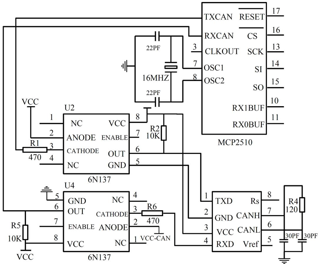
Fig. (4). The interface processing circuit in CAN bus.
