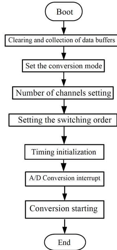
Fig. (8). The Initialization flow chart of CAN module in ARM.
