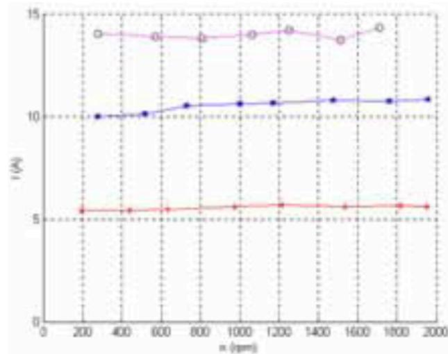
**Fig. (9).** Load characteristics of Wheel motor in constant torque area.
