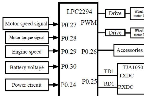
Fig. (3). The hardware circuit diagram in nodes of wheel motor.
