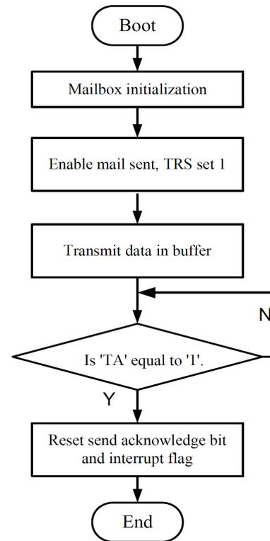
Fig. (7). The flow chart of transmission in CAN data.
