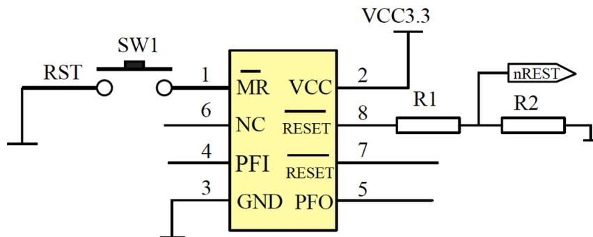
Fig. (5). The circuit schematic diagram inwatchdog and Reset.
