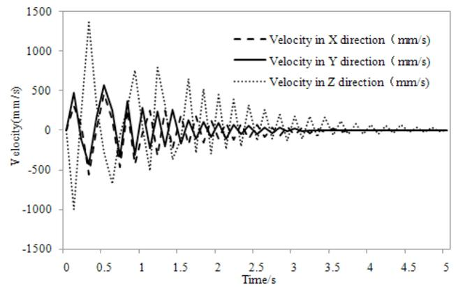
a) Vibration velocities in three directions of X, Y, Z
