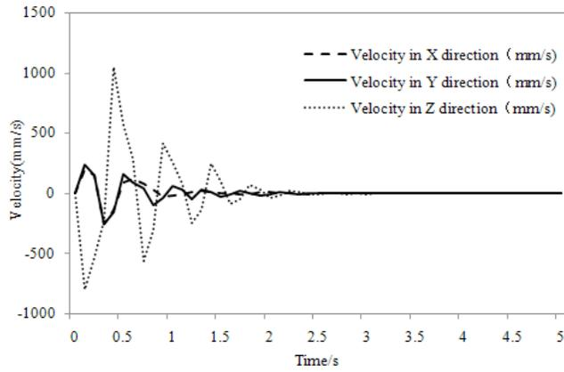
a) Vibration velocities in three directions of X, Y, Z
