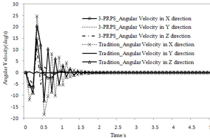
b) Comparison on the vibration angular velocities of the two reduction vibration devices in three directions of X, Y, Z.
