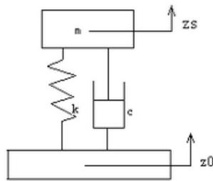
Fig. (1). Diagram of the reduction vibration mechanism inside the seat.
