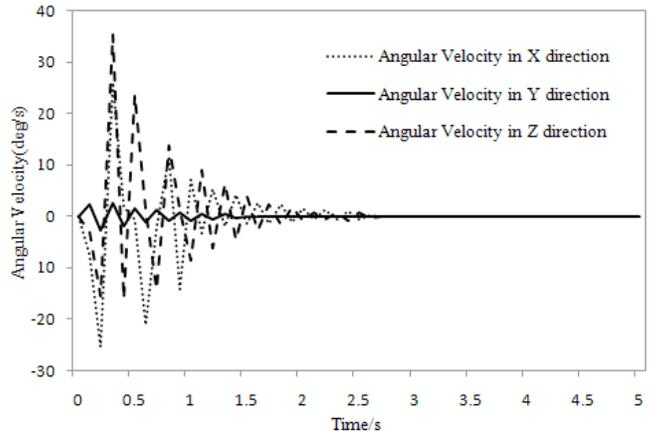
b) Vibration angular velocities in three directions of X, Y, Z
