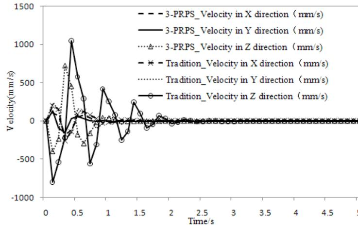
a) Comparison on the vibration velocities of the two reduction vibration devices in three directions of X, Y, Z
