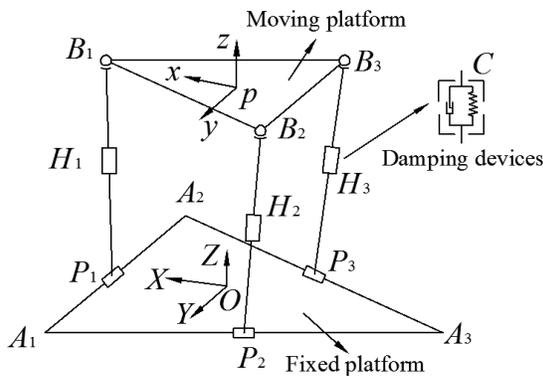
Fig. (4). Simple expression of 3-PRPS parallel mechanism.
