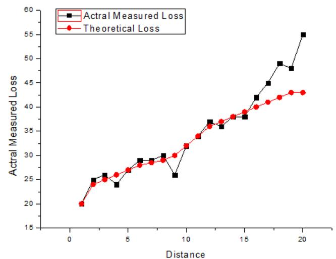
Fig. (6). The relationship between signal attenuation and distance.
