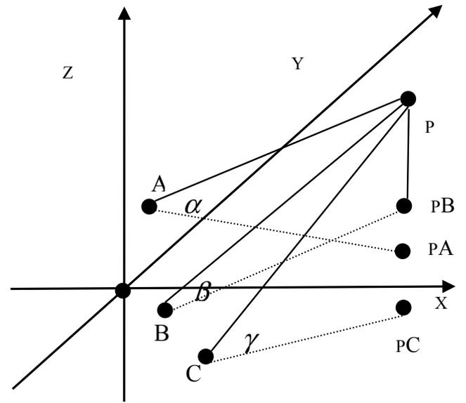
Fig. (4). Schematic positions of beacon nodes and unknown nodes in three dimensional space.
