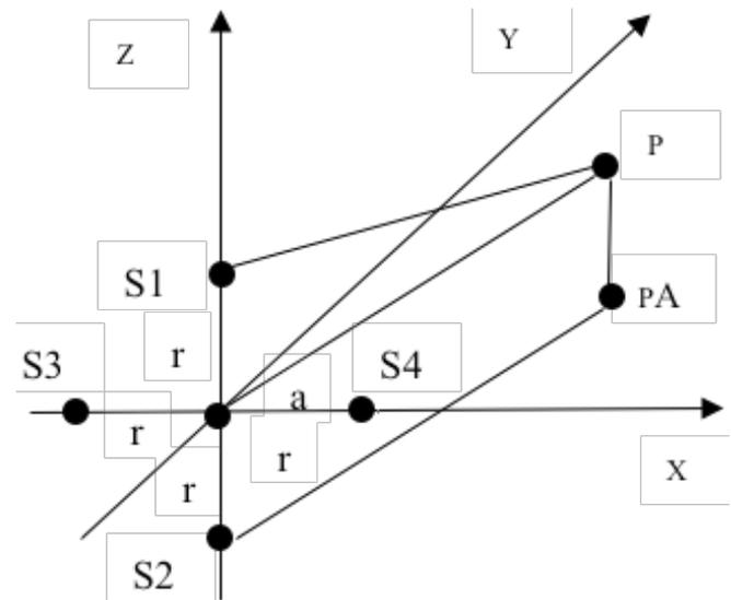
Fig. (3). Schematic positions of beacon nodes and unknown nodes.
