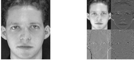
Fig. (2). One level 2D-DWT for an image from ORL.
