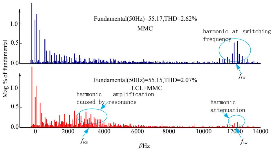
Fig. (8). FFT Analysis of Output Current.
