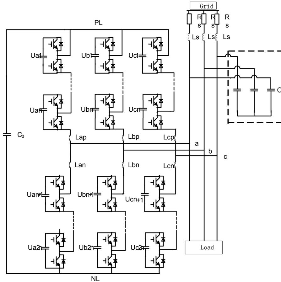
Fig. (1). Basic Structure of MMC-STATCOM.
