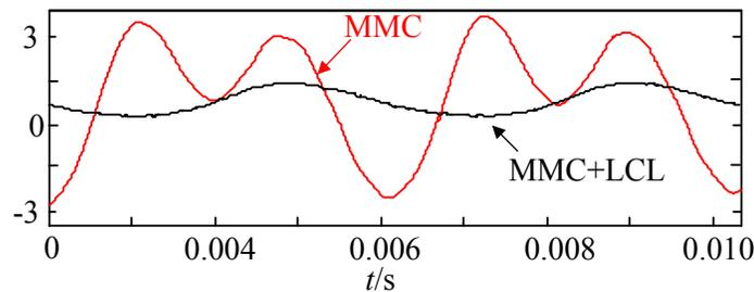
Fig. (9). Effect of Circulating Current Suppressor.
