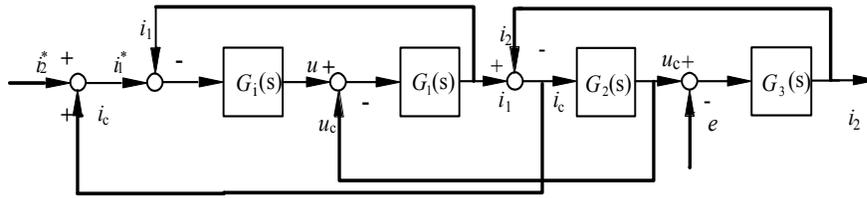
Fig. (5). Active Damping Strategy Based on Filter Capacitor Current.
