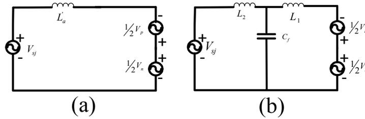
Fig. (2). Equivalent Circuit of A-phase MMC-STATCOM.
