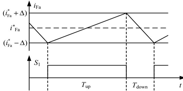
Fig. (4). Maximum Fluctuation of Current.
