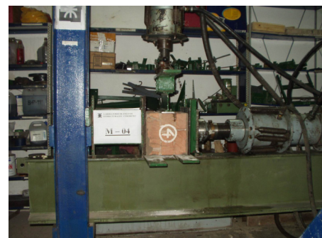
Fig. (6). Test set-up of combined compression and shear test of masonry.
