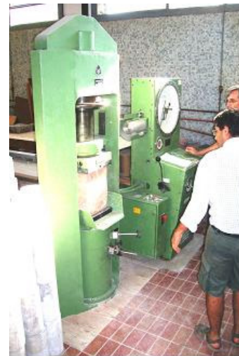
Fig. (5). Test set-up of the compression test.
