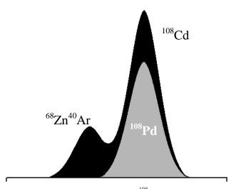
Fig. (1). Interferences profile on mass <sup>108</sup>Pd at medium resolution mode ( $m/\Delta m$ =3000).
