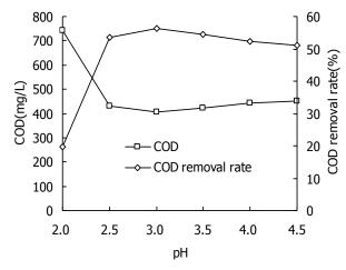
Fig. (1). The effect of pH value on COD removal.
