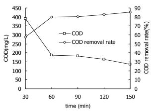
Fig. (7). The effect of reaction time on COD removal.
