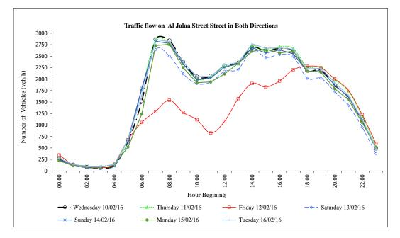
Fig. (4). Traffic flow distributions on al Jalaa street in both directions.
