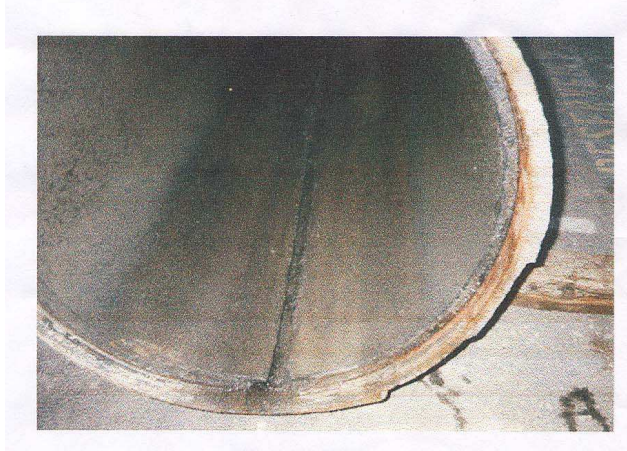
Fig. (1). The groove developed at the invert of the pressure main in Vancouver [6].
