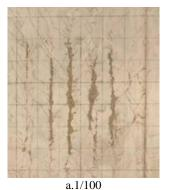
Fig. (9). Failure behaviors of SW1 at three drift ratios.
