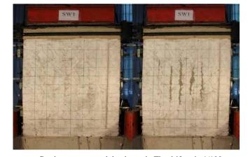
a. Crack pattern at peak loadb. The drift ratio 1/100Fig. (8). Failure process and pattern of SW1.
