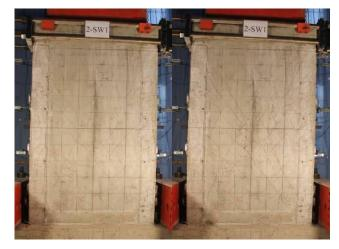
a. Crack pattern at peak load b. The drift ratio 1/70Fig. (7). Failure process and pattern of 2-SW1.
