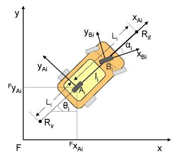
Fig. (1). Schematic of the vehicle.
