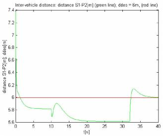
**Fig. (9).** Evolution of the inter-vehicle distance  $S_1P_2$  time (green line); Desired inter-vehicle distance during straight line motion of the leader:  $d_{des} = 6m$  (red line);  $L_1 = L_2 = 4m$ .
