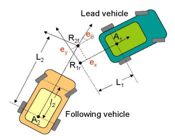
Fig. (2). System configuration for autonomous following.
