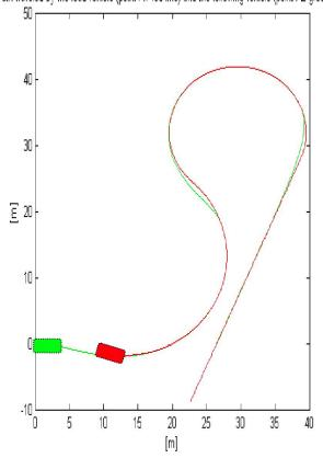
Fig. (6). A planar path drown by the vehicle guide points (the midpoints of the rear vehicle axles); red line (point  $A_I$ , lead vehicle), green line (point  $A_2$ , following vehicle),  $L_1=L_2=4m$ ;  $d_{des}=6m$ .
