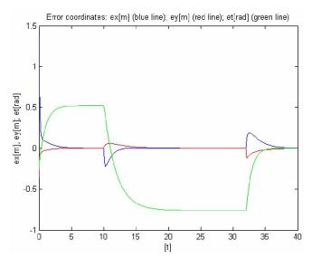
**Fig.** (7). Evolution of the error coordinates in time:  $e_x(t)$  (blue line);  $e_y(t)$  (red line);  $e_{\theta}(t)$  (green line);  $L_1 = L_2 = 4m$ ;  $d_{des} = 6m$ .
