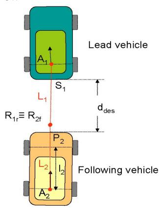
Fig. (5). Desired inter-vehicle spacing.
