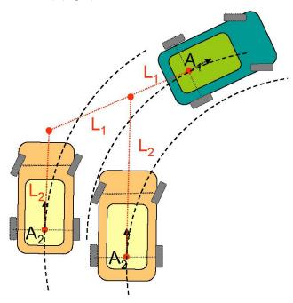
**Fig. (3).** Circular motion with  $L_1 \neq L_2$ .
