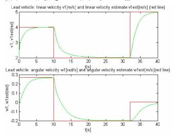
Fig. (8). Evolution in time of the lead vehicle velocities estimates  $(\hat{v}_{A1},\hat{\omega}_1)$  (green line); lead vehicle actual velocities  $v_{AI}$  and  $\omega_I$ (red line);  $L_1 = L_2 = 4m$ ;  $d_{des} = 6m$ .
