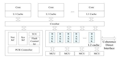
Fig. (1). Architecture of FT-8 processor.
