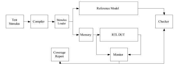
Fig. (2). FT-8 processor full-chip level simulation-based RTL verification platform.
