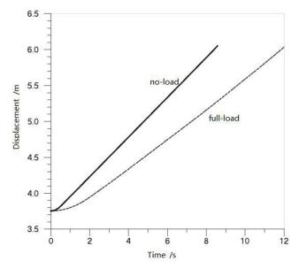
Fig. (13). The boom cylinder displacement curve in the lifting process.
