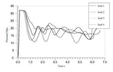
Fig. (18). The pressure change of the arm cylinder in different load conditions.
