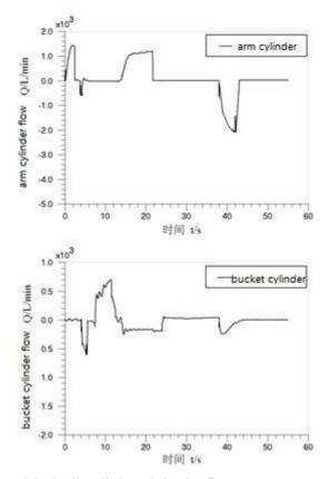
Fig. (23). Each hydraulic cylinder rod chamber flow curve.
