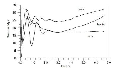
Fig. (20). The pressure curve of each hydraulic cylinder in the horizontal pushing condition.
