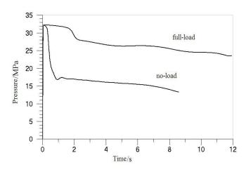
Fig. (15). The boom cylinder pressure curve in lifting process.
