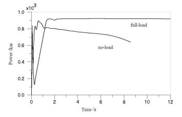
**Fig. (16).** The power consumption curve of the hydraulic pump in lifting process.
