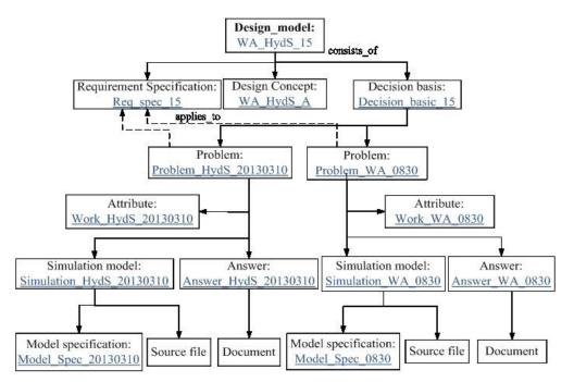
Fig. (3). A design model of the hydraulic system of the working device of the excavator.
