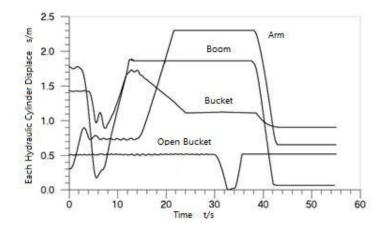
Fig. (22). Each hydraulic cylinder displacement curve.
