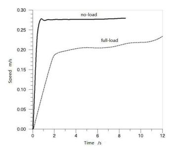
Fig. (14). The boom cylinder speed curve in the lifting process.
