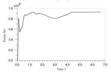
Fig. (21). The power consumption curve in the horizontal pushing condition.
