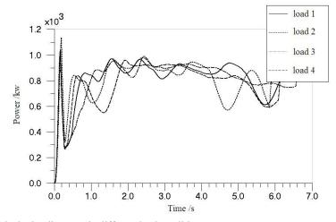
Fig. (19). The power change of the hydraulic pump in different load conditions.
