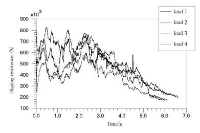
Fig. (17). EDEM digging resistance in different dipping depth.
