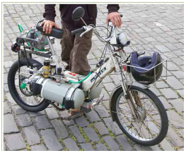
Fig. (1). Air powered moped.
