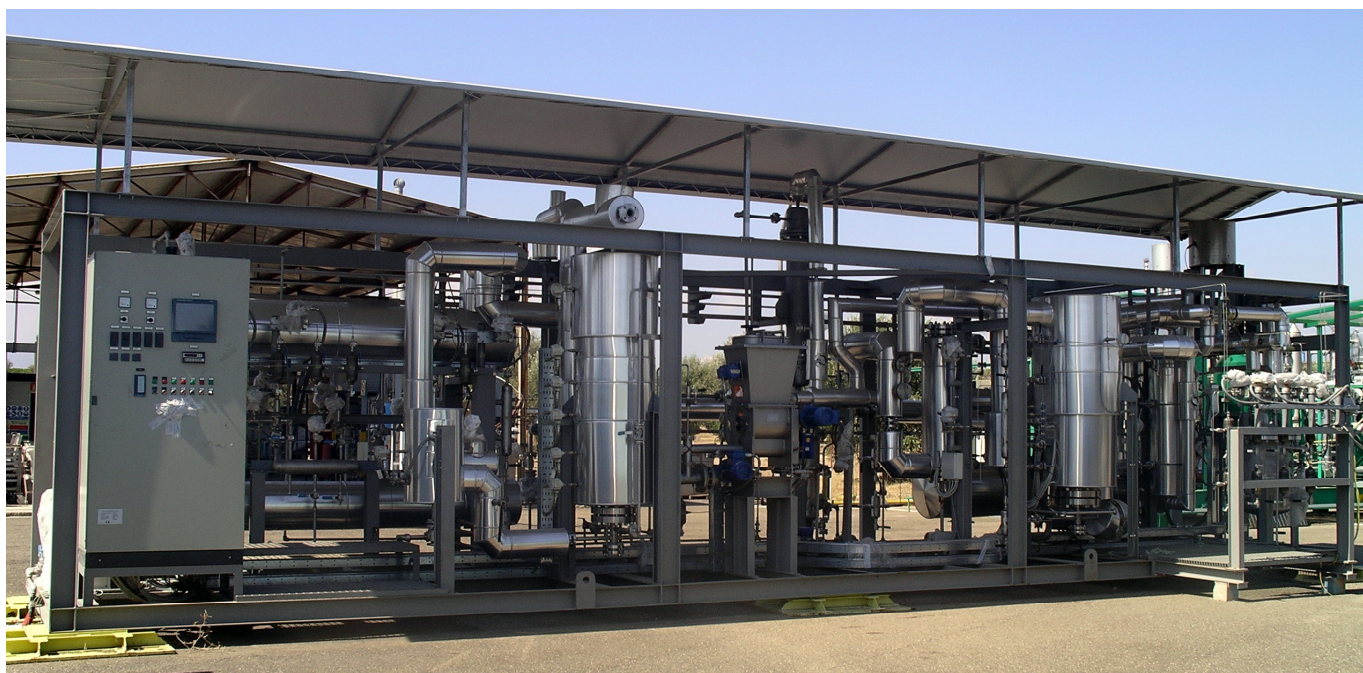
Fig. (4). Pilot plant for residues thermoconversion into hydrogen enriched gas [16].
