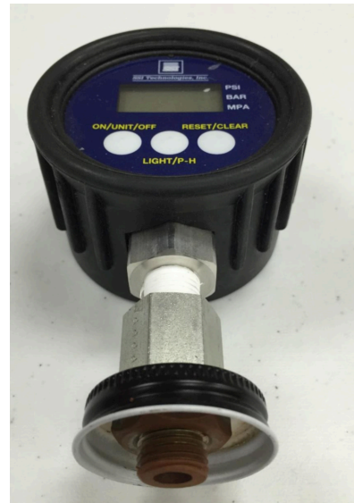
Fig. (5). Detail of pressure gauge sensor attachment to a screw-on container cap.
