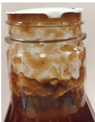
Fig. (6). Convex seal resulting from excessive headspace pressure due to the liquid nitrogen dose.
