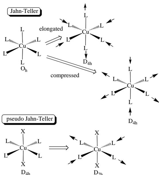
**Fig. (1).** Schematic representation of typical Jahn-Teller ( $O_h$ ) and pseudo Jahn-Teller ( $D_{4h}$ ) distortion of  $\text{Cu}^{\text{II}}$  complexes.
