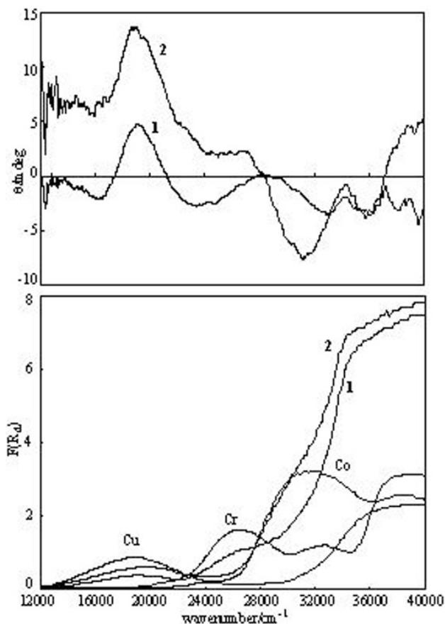
**Fig. (4).** [above] Solid state CD spectra in KBr pellets and [below] diffuse reflectance spectra of **1**, **2**, and [Cu(chxn)<sub>2</sub>](ClO<sub>4</sub>)<sub>2</sub> (**Cu**), K<sub>3</sub>[Cr(CN)<sub>6</sub>] (**Cr**), and K<sub>3</sub>[Co(CN)<sub>6</sub>] (**Co**).
