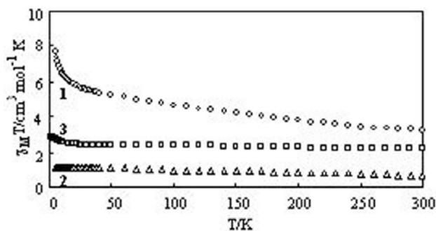
**Fig. (6).** The  $\chi_M T$  vs  $T$  plots at 5-300 K under 0.5 T for 1-3.
