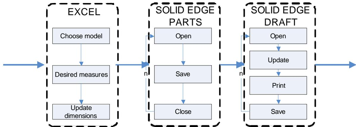
**Fig. (6).** General implementation architecture for flexible design of lockers.
