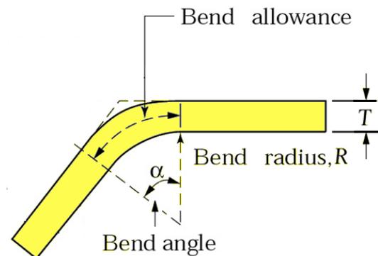
Fig. (3). Neutral axis in bending operations.
