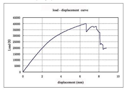
Fig. (16). Load - displacement curve of the aviation aluminum alloy flange by the tensile test.
