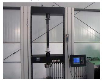
Fig. (8). Composite material flange tensile test.
