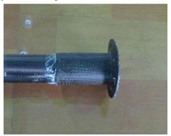
Fig. (7). Advanced composite material flange.
