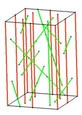
Fig. (2). Schematic illustration of the fiber structure of the threedimensional braiding.
