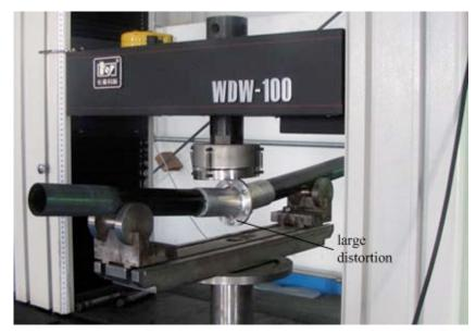
Fig. (18). Deform of the aviation aluminum alloy flange by the bending test.
