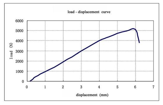
Fig. (13). Load - displacement curve of the composite material flange by the bending test.
