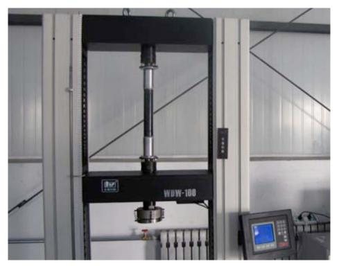
Fig. (14). Aviation aluminum alloy flange tensile test.
