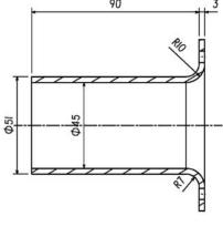
Fig. (3). Physical dimension of the flange.
