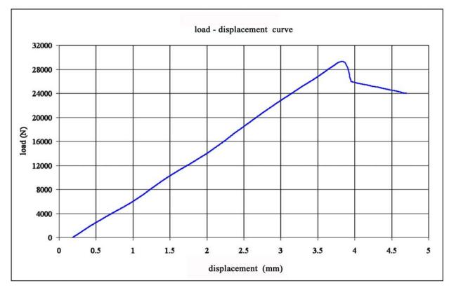
Fig. (10). Load - displacement curve of the composite material flange by the tensile test.
