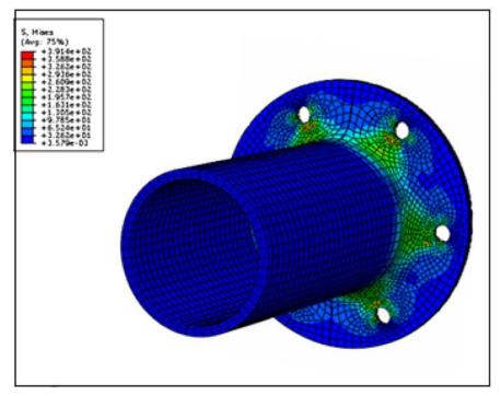
Fig. (20). Stress nephogram of flagne by the tensile test.
