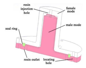
Fig. (5). Half sectional view of the mold.
