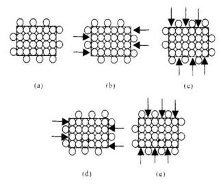
Fig. (1). The theory of four steps tabular braiding process of threedimensional braiding.
