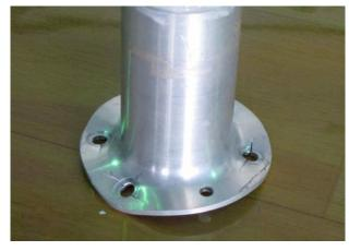
Fig. (15). Destroy of the aviation aluminum alloy flange by the tensile test.
