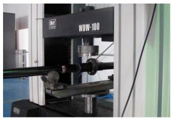
Fig. (11). Composite material flange bending test.
