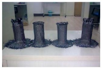
Fig. (4). Manufacture of the flange preform.
