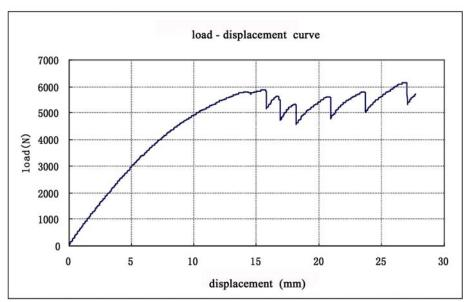
Fig. (19). Load - displacement curve of the aviation aluminum alloy flange by the bending test.
