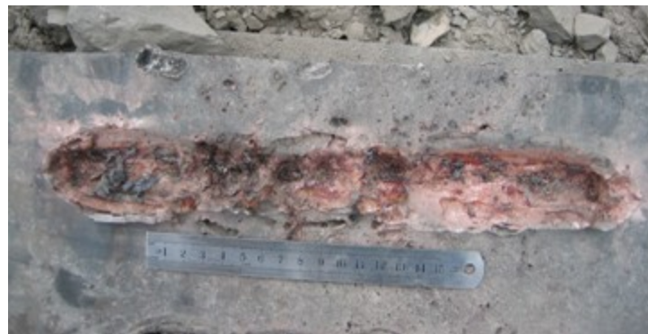
Fig. (3). Target result on the condition 10 times charge caliber stand-off.
