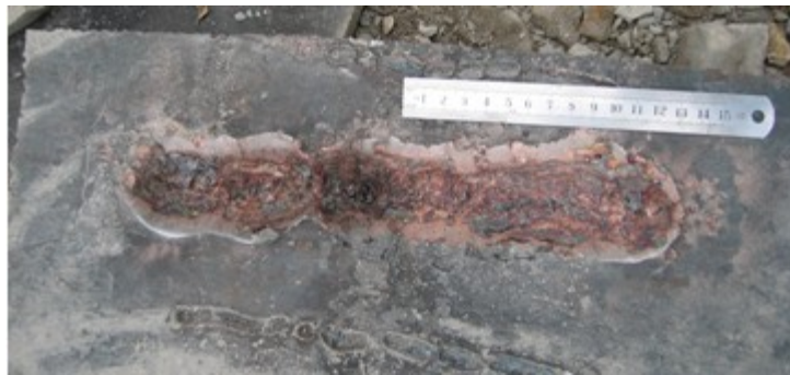
Fig. (2). Target result on the condition 5 times charge caliber stand-off.
