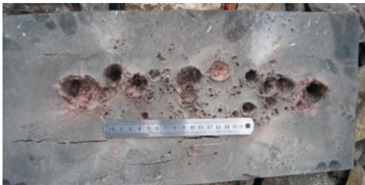
Fig. (4). Target result on the condition 20 times charge caliber stand-off.
