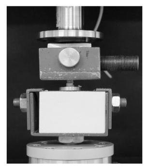
Fig. (2). Configuration of equipment for measuring screw pullout strength.
