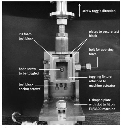
Fig. (1). Configuration of equipment for simulating screw toggling.
