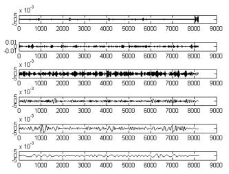
**Fig. (3).** Empirical mode decomposition of the whole tooth break signal.
