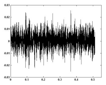
Fig. (2). The time domain of the whole tooth break signal.
