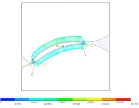
Fig. (5). Mathematical model of EMC characteristic section of the blade airfoil of gas-turbine engine compressor.
