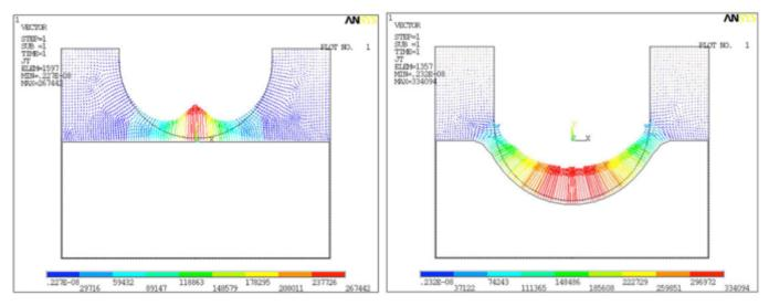
Fig. (3). Simulation results for a spherical electrode at the initial stage of machining and after 12 minutes for the material St20 on the electrolyte NaCl (20%).
