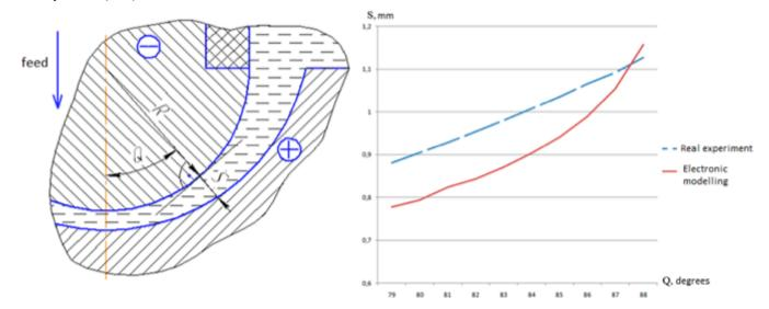
Fig. (4). Scheme of inter-electrode gap variation for EMC and the obtained results of comparison.
